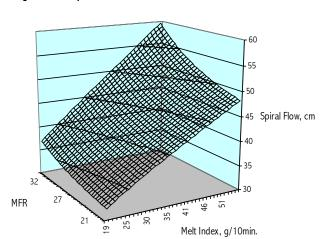
Figure 2. Spiral Flow as a Function of Melt Index and MFR
