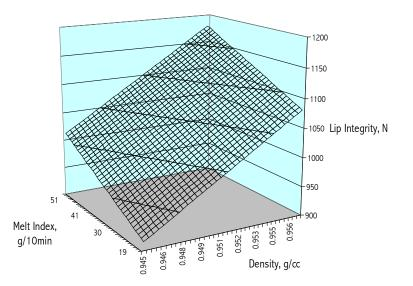
Figure 4. Lip Integrity as a Function of Density and Melt Index
