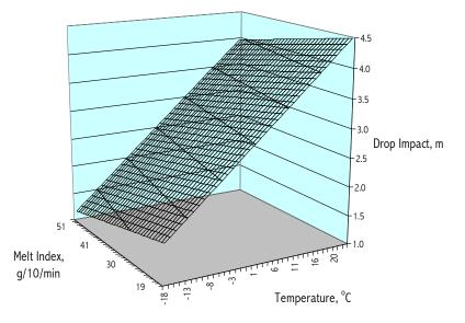
Figure 5. Drop Impact as a Function of Melt Index and Temperature
